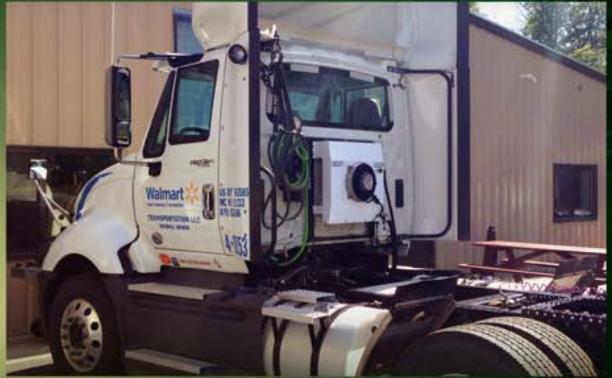
INTEGRATED PRIMARY A/C CONDENSER DAY CAB
